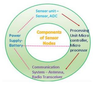
Figur3 –Sensor nodes components
