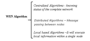
Figure 4- WSN algorithm characteristic approach
